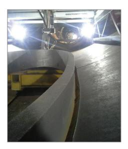
MCM machines perform precise multi-surface oxy-fuel cutting and beveling. Which is then followed by ideal workpiece fit-up and high quality SAW welding.
