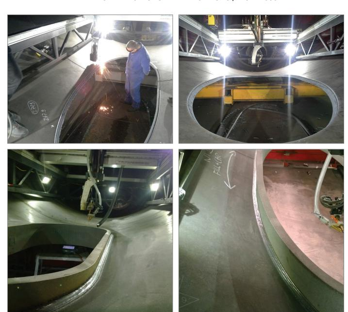
MCM door frame scanning, oxy cutting/beveling and SAW welding / One-man operation.
